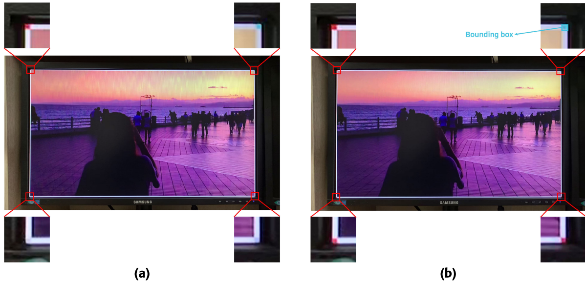
FIGURE 6. Received reference frame. (a) Sampling ratio: R_{rx}/R_{tx} = 120/60 = 2 . (b) Sampling ratio: R_{rx}/R_{tx} = 120/40 = 3 .
