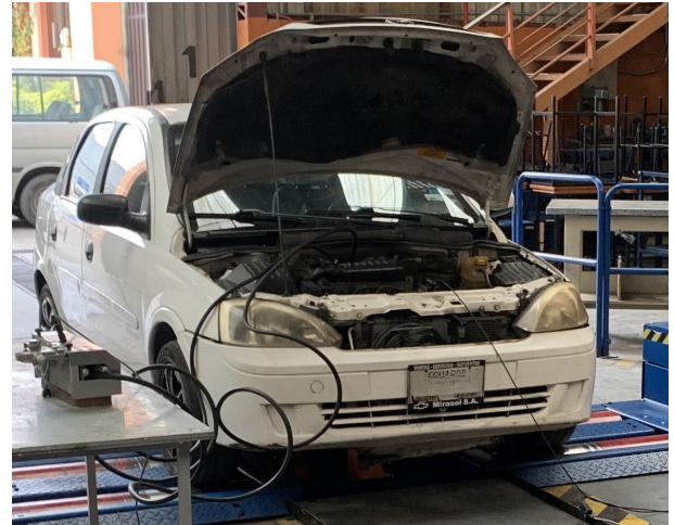
FIGURE 1. Car and test engine used for fault data acquisition.
