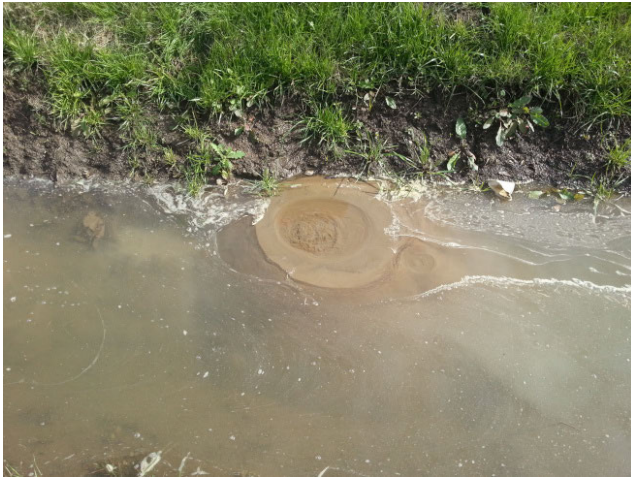
FIGURE 2. Example of sand boil in a levee system collected by the army corps of engineers in the new orleans district.
