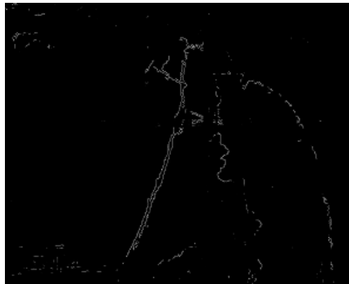
(a) Pseudo crack removal effect of MEMS devices image (curved crack)
