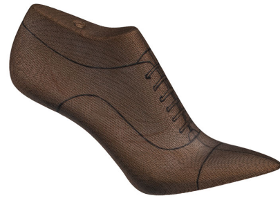
FIGURE 7. Shoe last digitalization. High-quality digitized triangle mesh (100.000 triangles) together with the texture applied. Below, the texture image with the pictures of all the shoe last parts.
