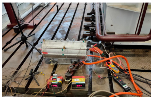
FIGURE 27. No-load test site.
