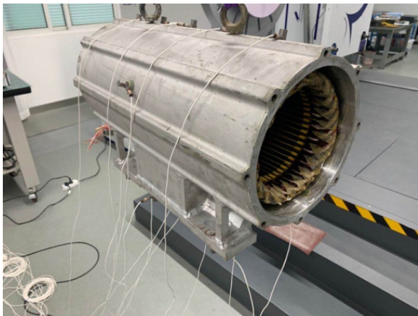
FIGURE 24. Modal test of the stator structure.
