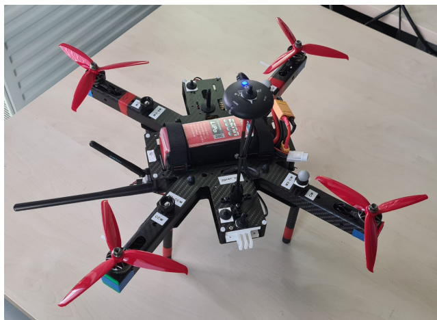
FIGURE 14. twinFOUR SCIENCE quadcopter equipped with a mounted battery (center, red), GPS antenna (with blue LED light), antenna for telemetry (left, small ant.), WiFi antenna (left, long ant.), and one IR-reflective marker for the mocap-system (right, small gray bulb).
