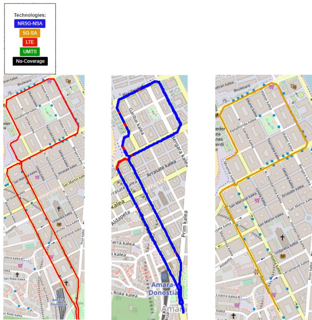
FIGURE 17. Coverage for LTE, 5G NSA, and 5G SA.
