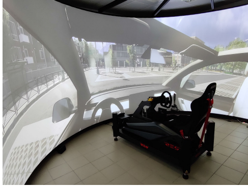
FIGURE 1. Vehicle driving simulator in the Autonomous Driving Laboratory of the University of Trento (Italy). The simulator uses real-time hardware to implement the presented VS model.
