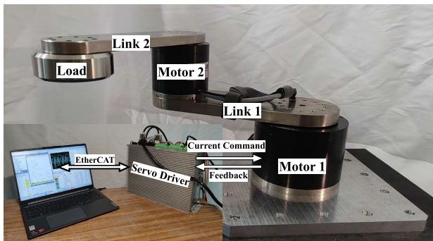
FIGURE 12. Experimental platform of the DDSCARA.
