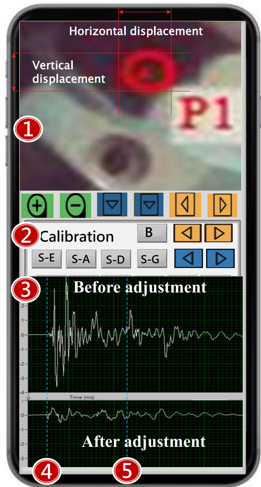
FIGURE 13. The vibrations measured by the high-speed camera and the accelerometers.
