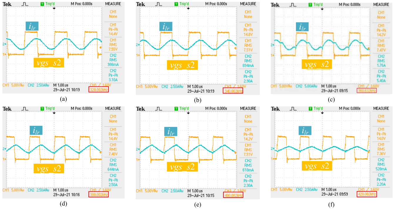
FIGURE 13. The waves of i_{Lmeq} at different operational frequency f_s .
