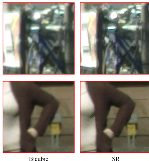
FIGURE 9. The examples of upscaled image regions that have false positives by SR. These images are the results of x4 upscaling using Bicubic and SR. The top images represent a region of the original image size at 48 \times 48 , while the bottom images represent a region of the original size at 64 \times 64 . We can see that the SR images are clear but have unnatural edges compared to Bicubic ones.
