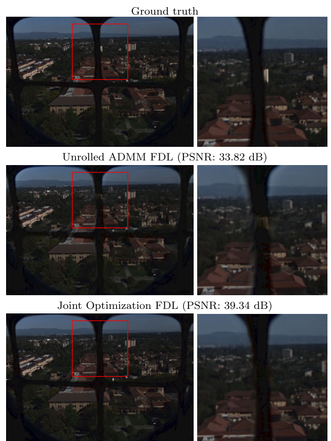
FIGURE 4. Example of an occluded region in the light field occlusion 36 eslf. The middle row illustrates the transparency artifacts with the FDL model in occluded regions: a building is visible through the grid of a window. These artifacts are reduced in the last row thanks to the learned view synthesis block of the proposed joint optimization.
