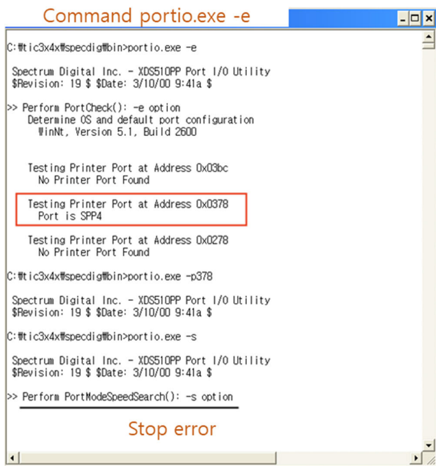
FIGURE 11. An error occurred while testing the status after successfully searching for the LPT's parallel port.
