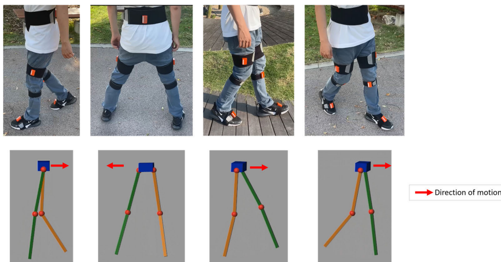
FIGURE 9. Comparison of the actual testing subject motion and simulation of the predicted joint angles. from left to right: backwards walking; sideways; ramp walking; zigzag walking.
