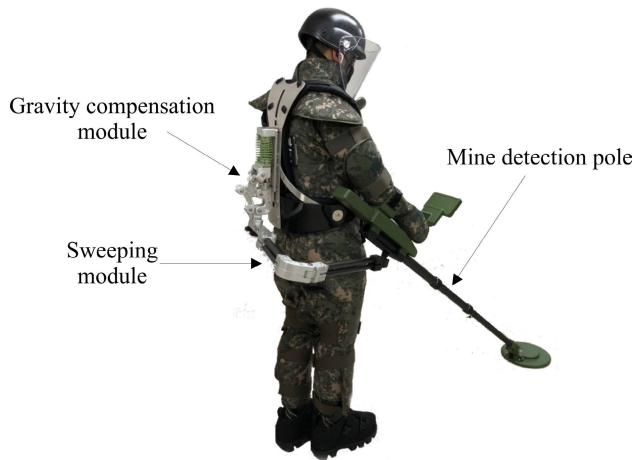
FIGURE 10. AX-Deminer forearm assistance worn by a mine-detection soldier.
