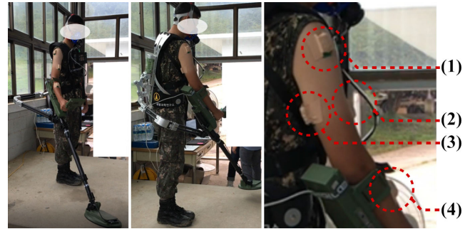
FIGURE 11. Experimental setup for the evaluation of the AX-deminer. For observing muscle activities during mine detecting motion, EMG sensors were attached to major muscles of the upper arm: (1) deltoid, (2) biceps brachii, (3) triceps brachii, and (4) brachioradialis muscles.
