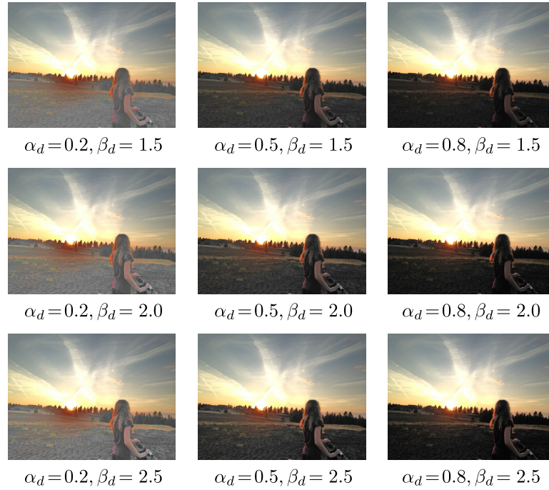
FIGURE 14. Changes in processing results when parameters \alpha_d and \beta_d are varied ( \alpha_b = 1.5 , n_p = 10 , \epsilon_{max} = 0.5 , and \sigma_{max} = 0.5 ).
