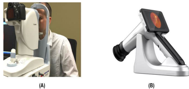
FIGURE 6. Fundus camera variants (A) Static (B) Mobile.
