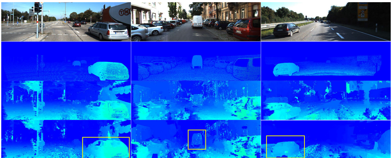
FIGURE 10. The disparity results on KITTI 2015 datasets. From top to bottom: the left view (reference image), real disparity map, MST, our method. From left to right: 000049_10, 000004_10, 000100_10.
