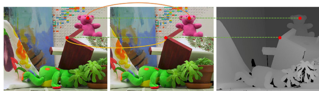
FIGURE 1. The Teddy in Middlebury [38]. From left to right: the left view (the reference image), the right view, the disparity map.
