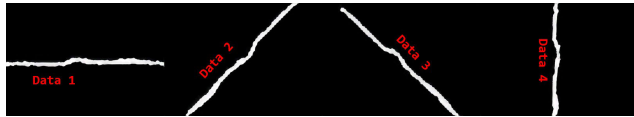
FIGURE 16. Generation of virtual cracks via data augmentation from input data (left to right : 0^\circ, -45^\circ, 45^\circ, 90^\circ ).
