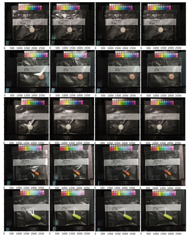
FIGURE 11. Some results of glare removal. The two leftmost images in each row depict the two captured input images from a test sample. The two rightmost images exhibit the results after applying glare removal to the respective input images.
