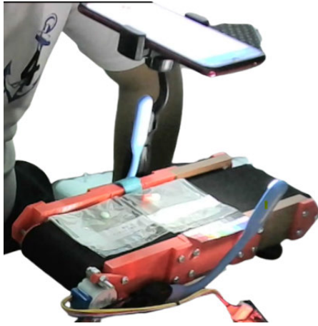
FIGURE 3. The developed apparatus for automatic image capturing of medication packages.
