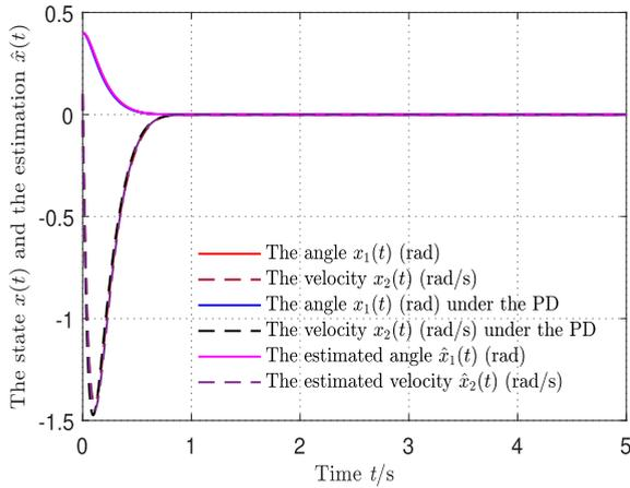
FIGURE 1. The angle and angular velocity stabilization curves.
