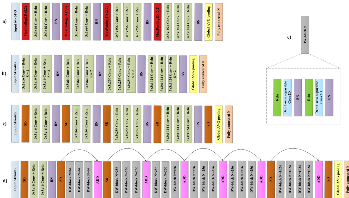
FIGURE 3. The proposed architectures for image classification: (a) CNN architecture with max-pooling (MP) for down-sampling, (b) CNN architecture with strided convolution for down-sampling (s refers to both the vertical and the horizontal strides), (c) CNN architecture with Depth-to-space (SD) for down-sampling, (d) CNN with depthwise separable convolution and SD for down-sampling, and (e) is the depthwise block (DW-block) (used in the architecture d) which consists of a single repetition of Relu followed by depth-wise separable convolution and batch normalization.
