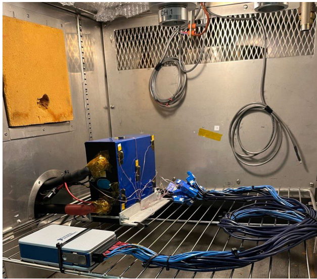
FIGURE 2. Battery setup inside the thermal chamber.
