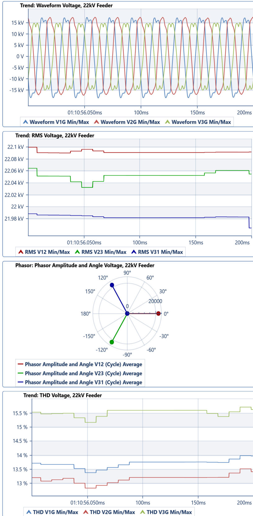
FIGURE 4. Harmonics PQD Condition – Real Field Data - 22kV Australian Distribution Feeder: Continuous L-G Voltage Waveform, RMS Voltage, Magnitude and Angle Voltage Phasors, THD Voltage.
