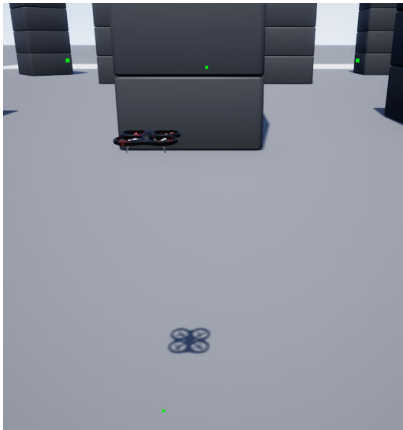
FIGURE 7. Drone setup. The four single-point laser distance sensors are depicted with green dots.
