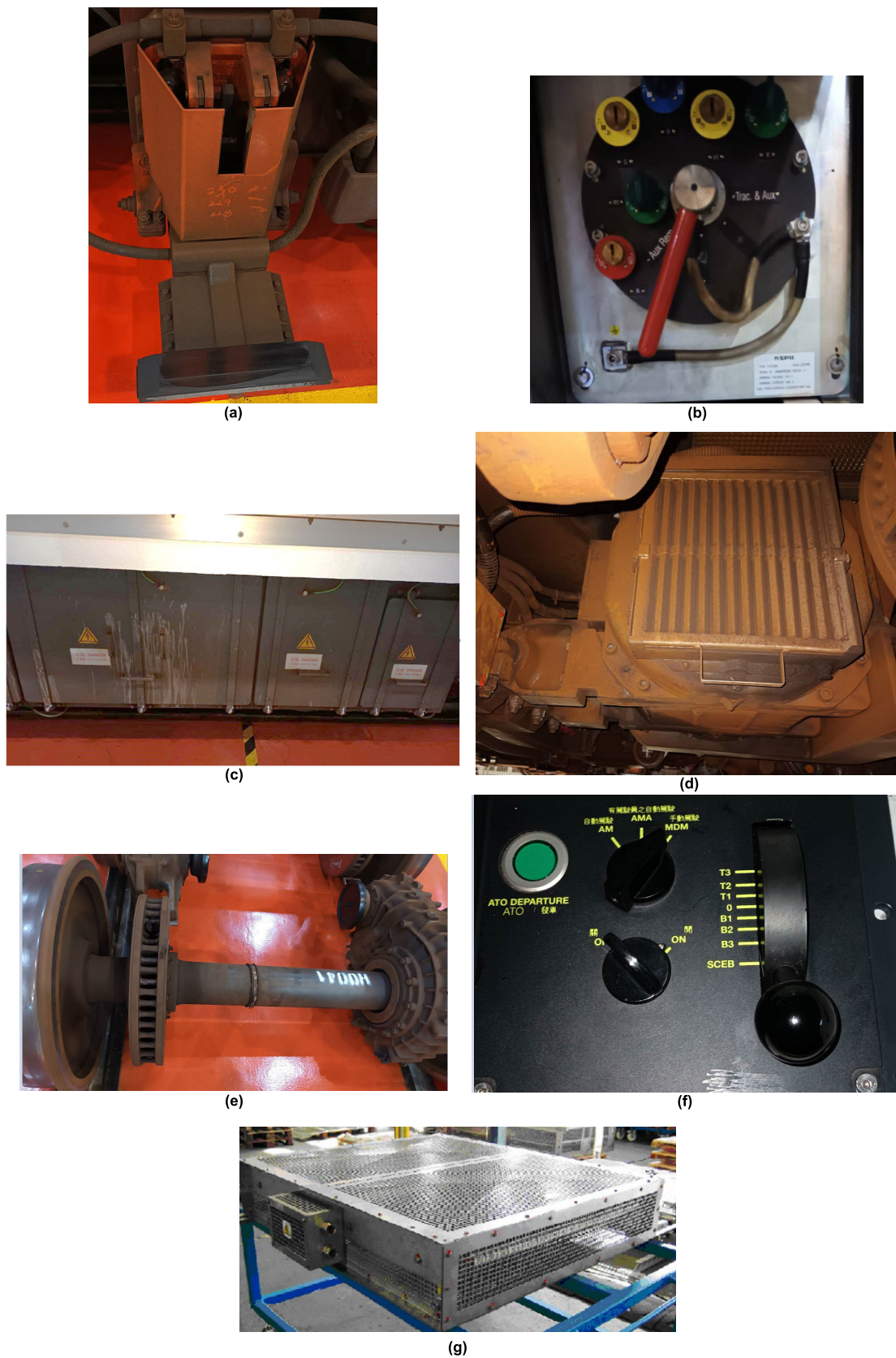
FIGURE 3. Essential components of a power car propulsion system: (a) current collector, (b) knife switch box, (c) line switch box and electrical equipment box, (d) traction motor, (e) wheel, (f) master controller, (g) line reactor.
