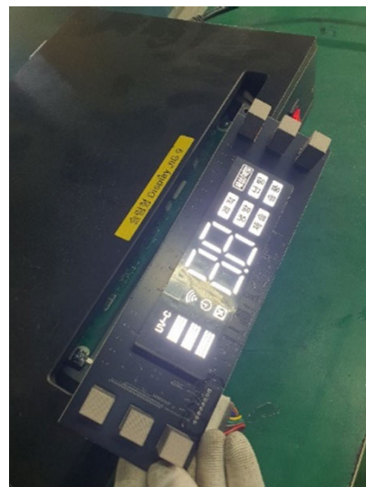
FIGURE 3. Power on status for lighting test.
