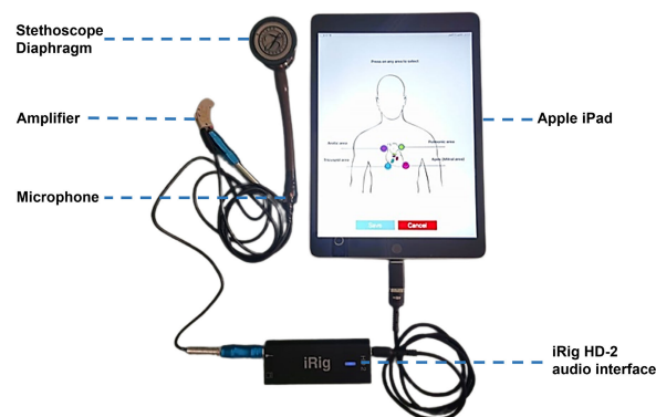
FIGURE 4. Developed In-house stethoscope.
