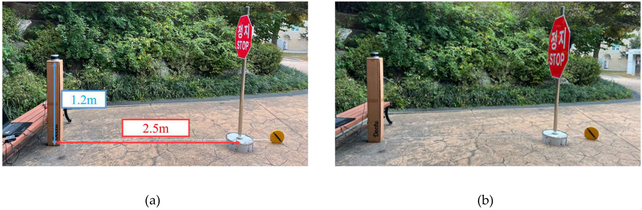
FIGURE 4. Reflection characteristic experiment: (a) diffuse reflector, (b) retroreflector.
