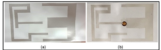
FIGURE 5. a) Printed RFID sensor structure (b) Printed RFID sensor structure with chip integration.
