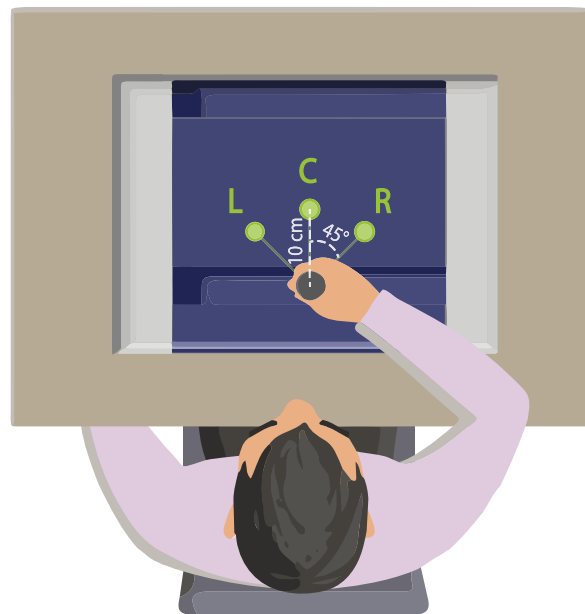
FIGURE 1. Experimental set-up. Participants were seated in front of H-Man, with the center of their sternum aligned with the center of the robot's workspace, where the starting position was located (gray). They had to grasp the robot's handle, which was moved by the robot to one of three possible target locations (green), located 10 cm from the starting position at 0° (central: C) and \pm 45^\circ (right: R, left: L) with respect to the participant's midline.
