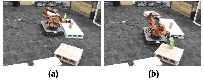
FIGURE 9. Robot in action to carry out the user's instructions. (a) :Execution of O_1 \in P_1 \rightarrow O_1 \in G_1 and O_0 \in P_0 \rightarrow O_0 \in G_0 . (b):Execution of O_1 \in G_1 \rightarrow O_1 \in G_3 and O_0 \in G_0 \rightarrow O_0 \in G_2 .
