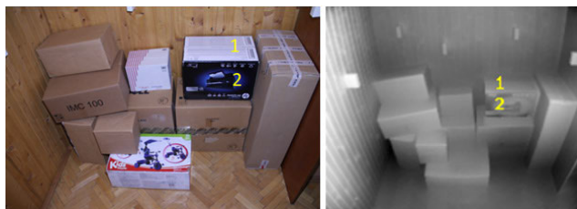
FIGURE 11. Photograph and distance map of a scene containing a package made of highly reflective material. The visible sides of the box are marked with 1 and 2. The edge between the sides is non-distinctive in the distance map.
