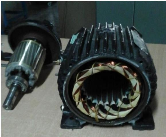
**FIGURE 9.** Components of conventional machine (3- $\Phi$ ).
