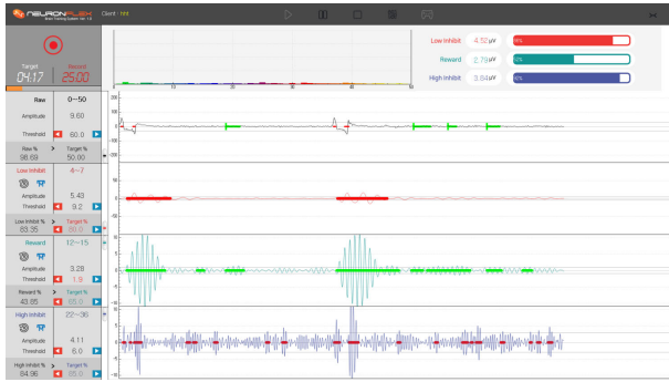
FIGURE 4. Decision of success and failure sections in theta wave (low inhibit), SMR (reward), and high beta wave (high inhibit).
