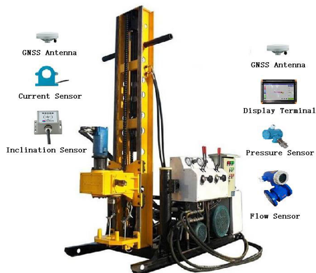
FIGURE 4. Schematic diagram of digital monitoring hardware sensors.
