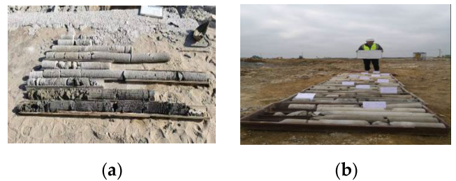
FIGURE 27. A core drilling and coring diagram of a rotary jet grouting pile: (a) Example of drilling coring; (b) Drill hole coring number.
