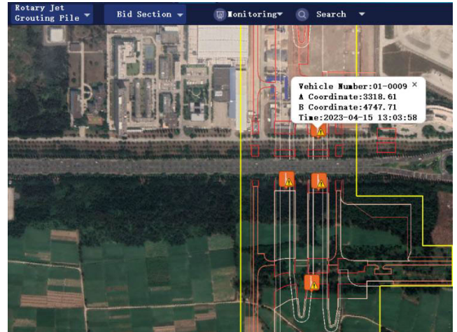
FIGURE 11. Digitally monitored position diagram of the rotary spray pile.
