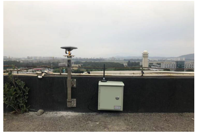
FIGURE 8. Installation diagram of GNSS positioning base station.
