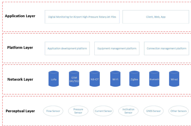
FIGURE 2. Architecture diagram of the internet of things.
