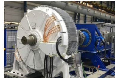
FIGURE 2. Magnetically geared generator for wind turbines.
