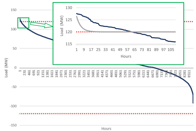
FIGURE 8. Load Duration Curve in blue of a 132kV line for one year. Calculation of the hours to be curtailed. The TC can be seen in grey in the zoom. Source: I-DE (Spanish DSO).
