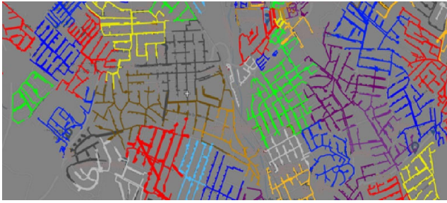
FIGURE 16. LV grid in the area of a single-family house. Each colour represents a different feeder. Source: i-DE (Spanish DSO).
