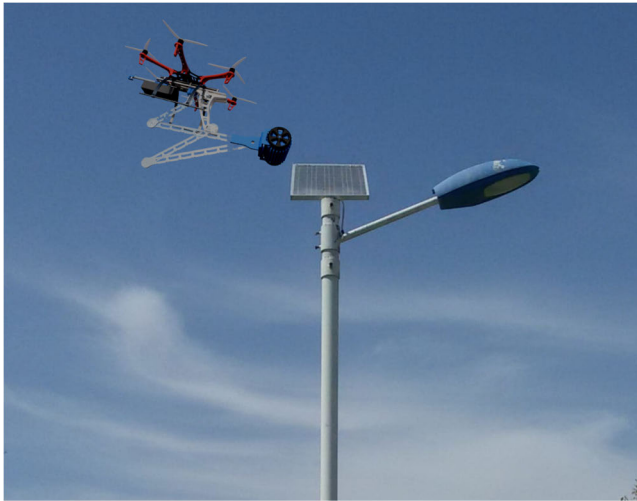
FIGURE 2. Proposed cleaning system positioned above solar panel light installed in a residential location.
