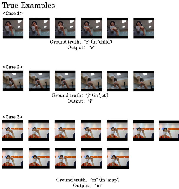
FIGURE 10. True case of air-writing recognition by three examples. The pictures on the upper row are the sequence of images corresponding to a particular letter in the action of drawing a word. The text on the middle row shows the actual correct character and the character output by the proposed method on the lower row, which is correct.
