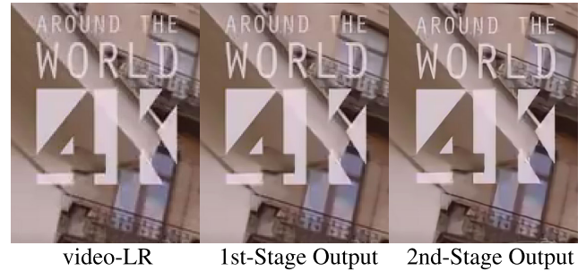
FIGURE 6. Results in the actual edge device. These images are the result of storing the actual HW output using Alpha 9 Gen-6 DTV SoC. The noise caused by compression was removed in the first stage, and the Super-resolution was well performed in the second stage.
