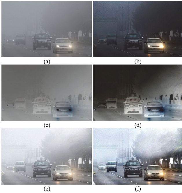
FIGURE 2. (a) Low-visibility images caused by haze; (b) Dehazed image of (a) obtained using DCP [1]; (c) Negative image of (a); (d) Dehazed image of (c) obtained using our dehazing algorithm; (e) Positive image of (d); (f) Final enhanced image of (a) obtained using the proposed framework.
