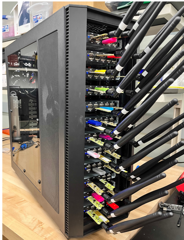
FIGURE 10. Front bank of USB hubs on the transmitter host machine with 20 Yard Stick One devices distributed throughout.
