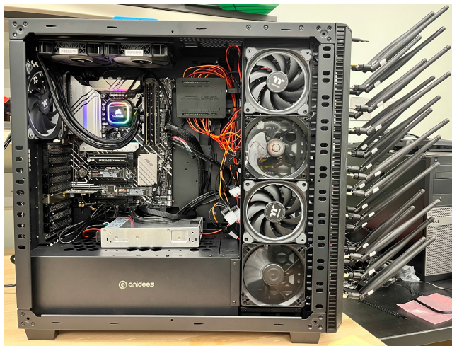
FIGURE 9. Side profile of the transmitter host machine with the side panel removed. The motherboard occupies the back of the case and the main PSU (not visible) is in the bottom compartment. On top of the bottom compartment is the auxiliary PSU, which is connected to the USB hub relays near the top-front of the case. The tip of the atmospheric probe is visible on the top front of the case above the bank of antennas.
