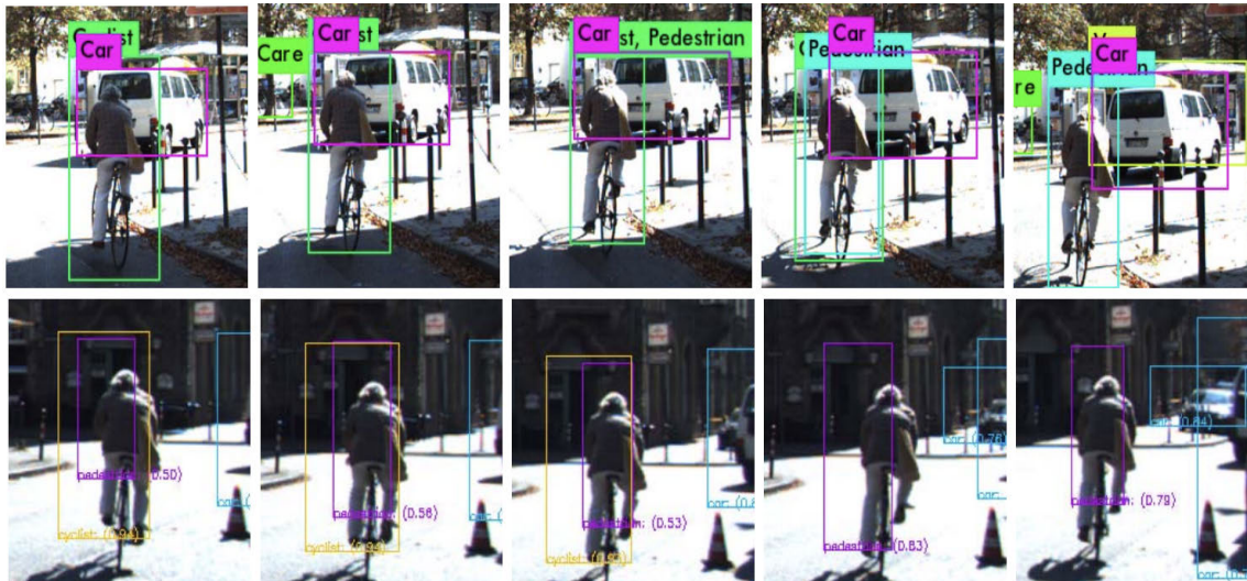
FIGURE 19. a) With high confidence (greater than 75%), YOLOv3 incorrectly labels the cyclist as a pedestrian; b) The possibility that YOLO will detect a cyclist varies from 0 to 75%.
