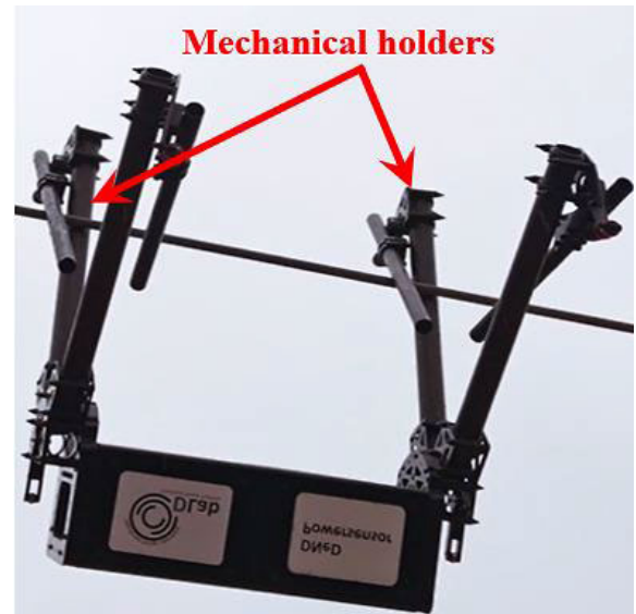
FIGURE 10. The mechanical holders of the drone's black box [18].
