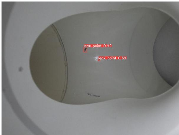
(c) YOLOv5s test results at the tee
