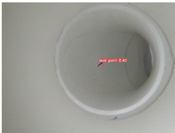
(e) test results of the YOLOv5s method at the joints of the two tubes
