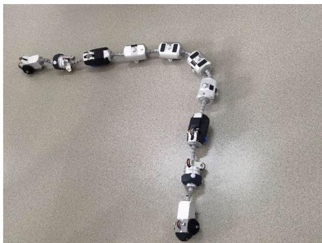
FIGURE 7. Robot for inspection in buried gas pipelines.
