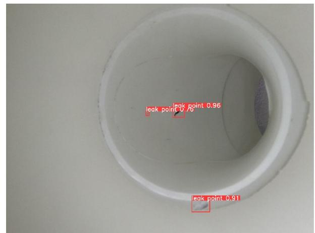
(f) test results of this paper's method at the joints of the two tubes
