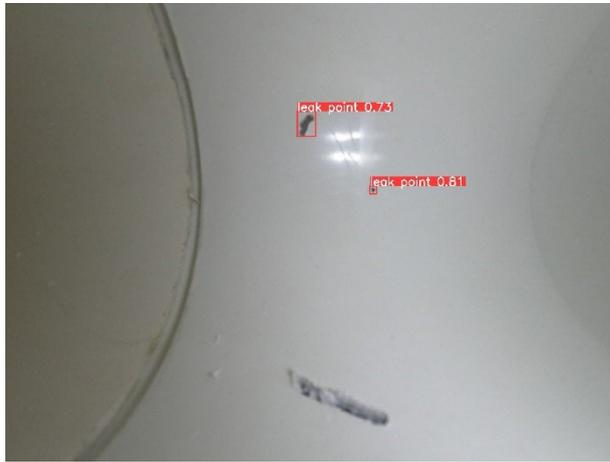
(a) detection results of YOLOv5s with holey structure and irregular shape leakage
