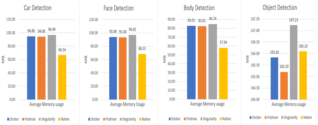
FIGURE 8. Average memory usage for different containers for computer vision application in wired-wired connection.
