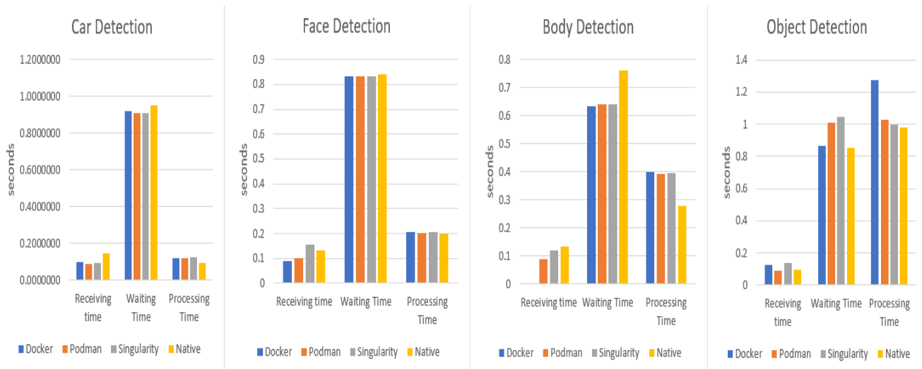
FIGURE 6. Average receiving, processing, and waiting time for different containers for computer vision application in wireless-wireless connection.
