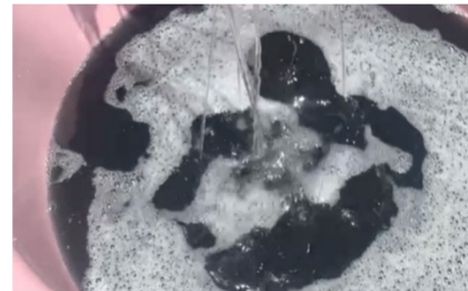
FIGURE 9. Turquoise insulation oil after 800 A arc fault.
